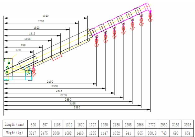
Notice: It is necessary to adjust the Rod according the capacity of load and boom distance.
